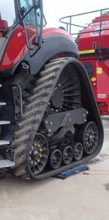
Figure 7: Use weigh cells to determine the maximum ballasted axle loadings for various operations. Once done, adjust tyre pressures accordingly. This is also important for the front tyres on half-tracked tractors, which can otherwise exert high pressures
