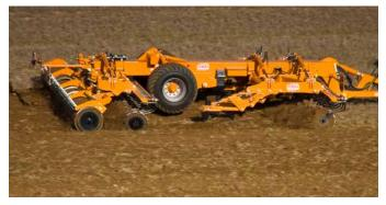
Figure 23. Typical high disturbance, deep non-inversion mixing action
