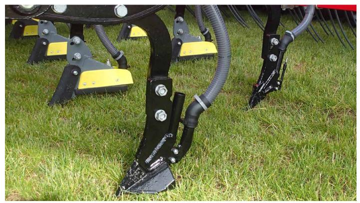
Figure 33. Alternative openers for a tine drill to modify the amount and degree of soil disturbance and drilling band width
