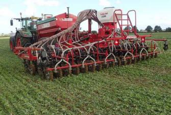
Figure 6. Cover crop established into a stubble with a relatively high-disturbance tine drill (top). Main crop drilled into a cover crop with a low-disturbance, disc-based drill (bottom). Both drilling modules can be mounted on the same leading hopper
