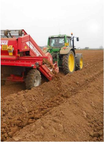
Figure 41. When destoning, monitor depth for improved work rates and fuel consumption
