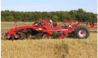
Figure 25: Shallow non-inversion tine and disc-based machine options
