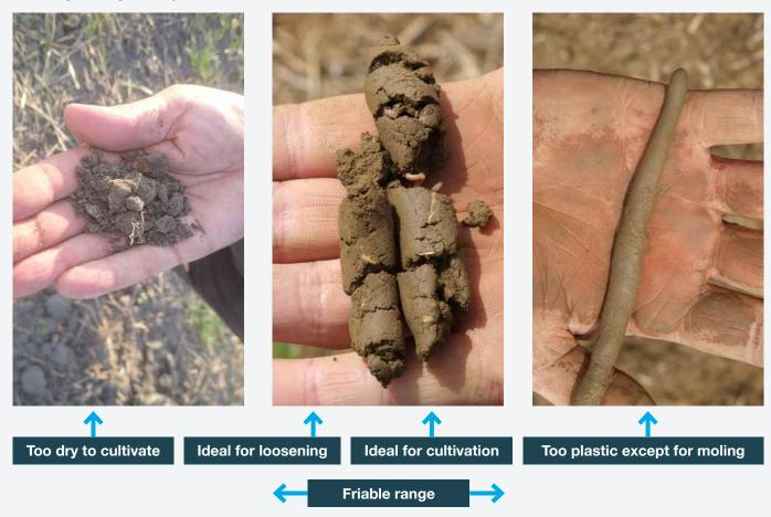
Fundamental moisture principles govern the interactions between soil and metal for all forms of cultivation: deep, shallow or reduced. Soil moisture content should be assessed to ensure it is appropriate for cultivation. To assess soil moisture, use a ribbon test on a sample from the soil surface and at cultivation depth.
