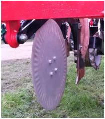
Figure 32. Examples of tine-based drills with leading discs. These enable effective operation in higher levels of residues and reduce soil disturbance
