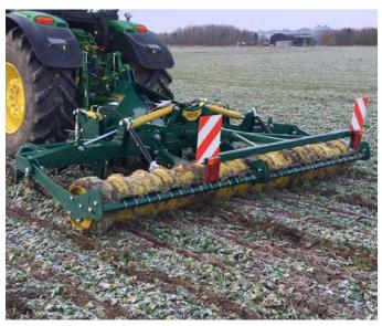
Figure 13. Soil loosening through a growing cover crop
