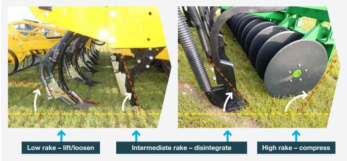
Fundamental principles of geometry govern the interaction of soil and metal.
