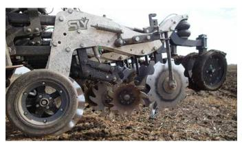
Figure 28. Specialised strip-till cultivation units prepare ground for later drilling
