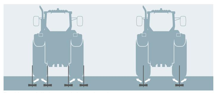
Figure 9. Loosen each side of permanent wheel-ways or along tracks
