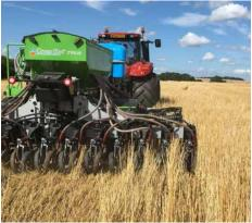
Figure 4. Long, anchored stubbles left by stripper heading (left) can be drilled with a suitable direct drill. Note: requires effective chaff spread
