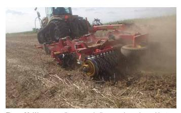
Figure 26. Wave-type discs on a shallow non-inversion cultivator
