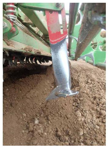
Figure 40. Option to loosen below the pick tines of a bed-former, aligned to the rows that will be planted next
