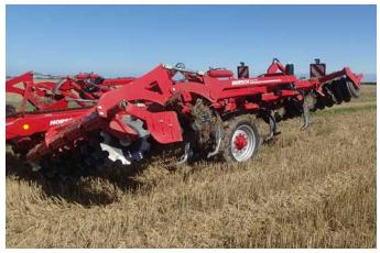
Figure 24. Lower surface disturbance, shallower discing machine option
